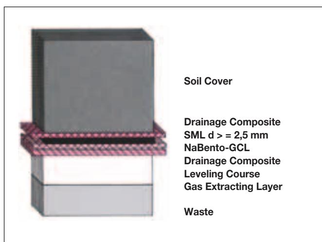
Capping system using geosynthetics
